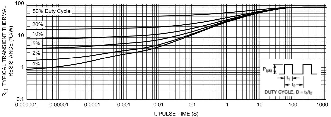
Figure 9. Typical Transient Thermal Response, Junction-to-Ambient for NRVTSA3100E
