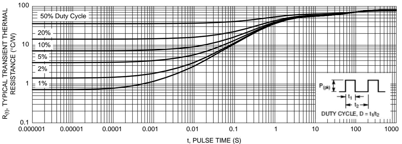
Figure 10. Typical Transient Thermal Response, Junction-to-Ambient for NRVTSAF3100E
