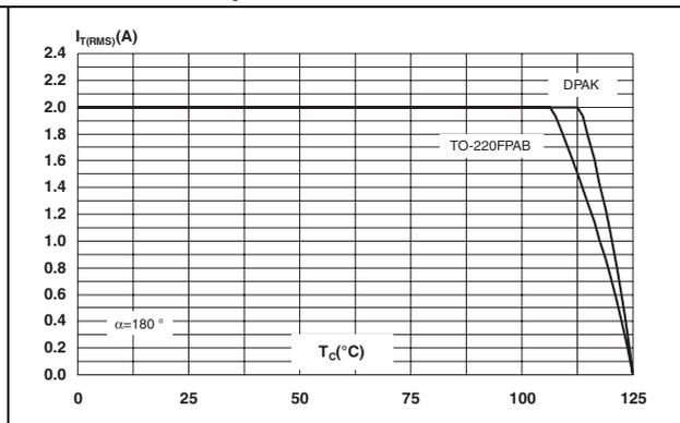
Figure 4. On-state rms current versus ambient temperature
