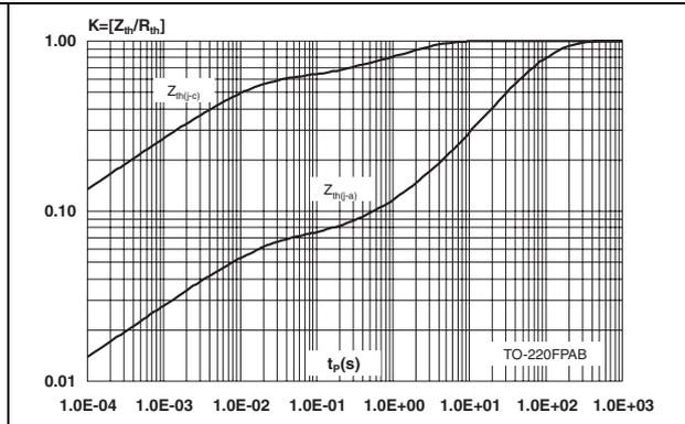
Figure 6. Relative variation of thermal impedance versus pulse duration DPAK
