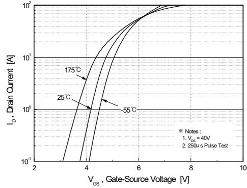
Figure 2. Transfer Characteristics
