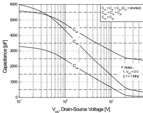
Figure 5. Capacitance Characteristics
