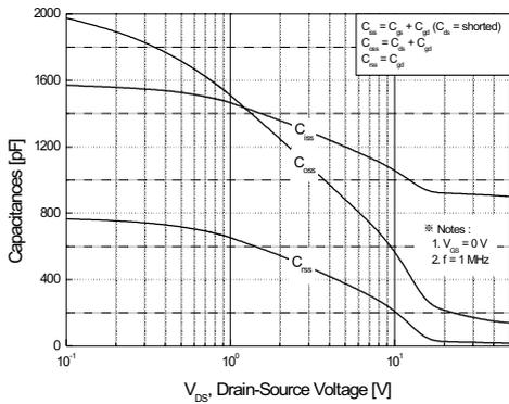
Figure 5. Capacitance Characteristics
