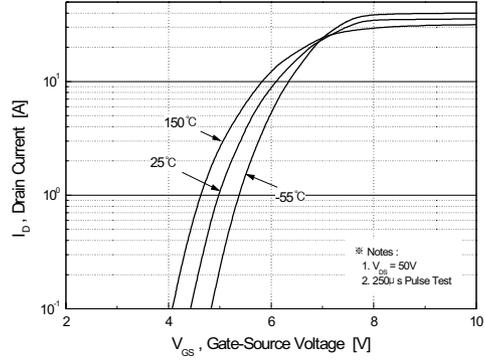
Figure 2. Transfer Characteristics
