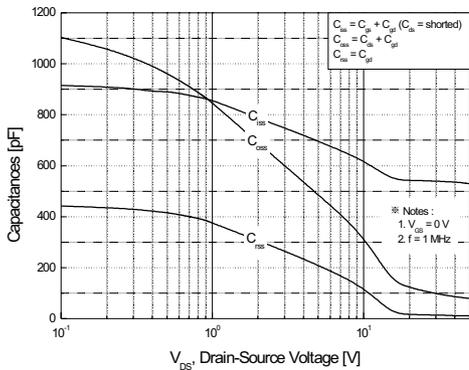
Figure 5. Capacitance Characteristics
