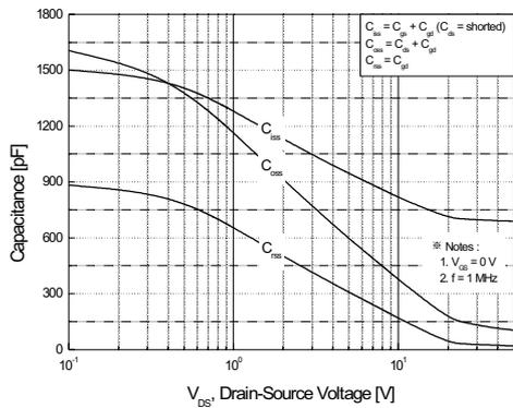
Figure 5. Capacitance Characteristics
