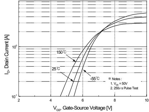
Figure 2. Transfer Characteristics
