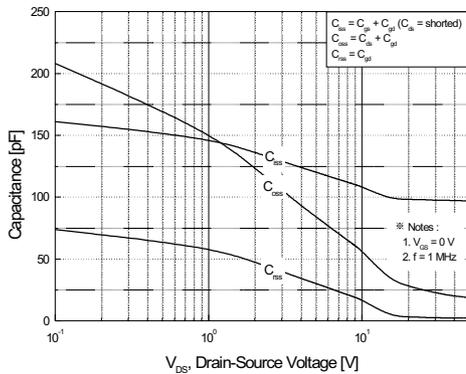
Figure 5. Capacitance Characteristics
