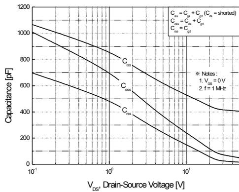
Figure 5. Capacitance Characteristics
