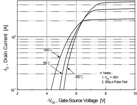
**Figure 2. Transfer Characteristics**
