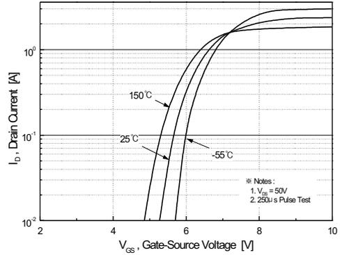
Figure 2. Transfer Characteristics
