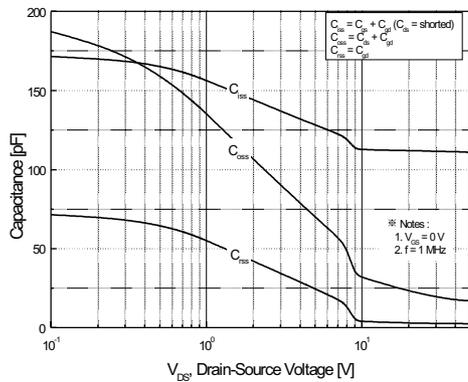
Figure 5. Capacitance Characteristics
