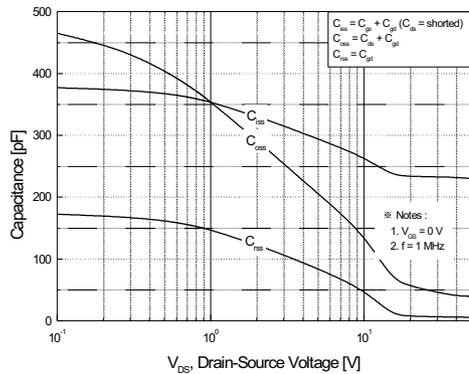
Figure 5. Capacitance Characteristics
