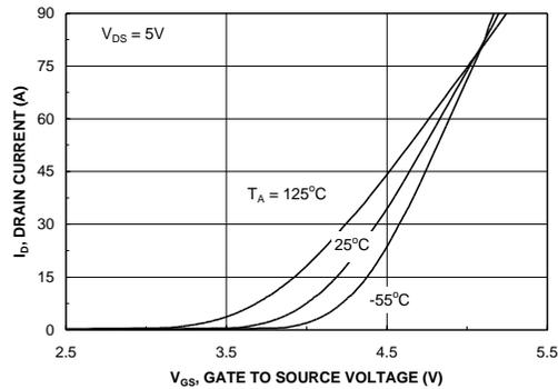
Figure 5. Transfer Characteristics.
