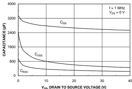
Figure 8. Capacitance Characteristics.
