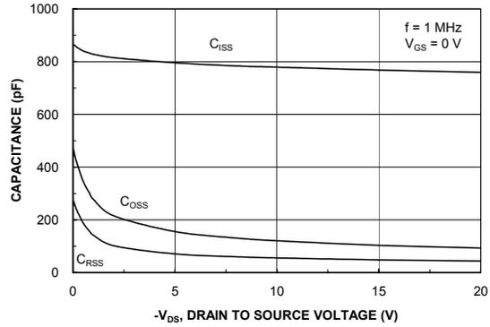
Figure 8. Capacitance Characteristics.
