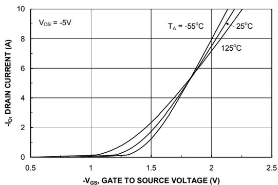
Figure 5. Transfer Characteristics.
