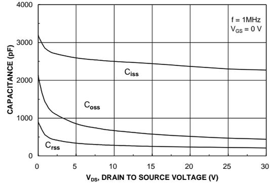
Figure 8. Capacitance Characteristics.
