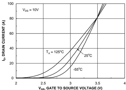
Figure 5. Transfer Characteristics.
