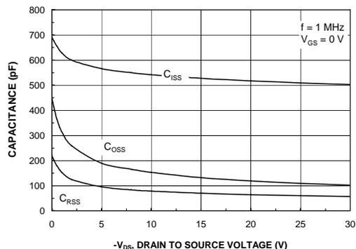
Figure 8. Capacitance Characteristics.
