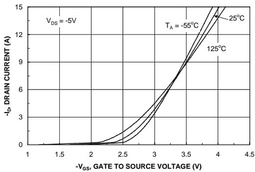
Figure 5. Transfer Characteristics.
