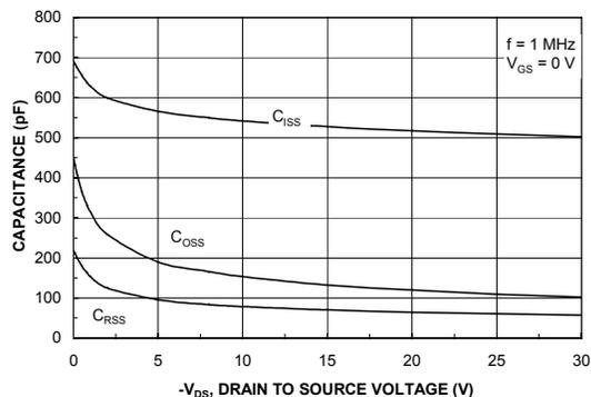
Figure 8. Capacitance Characteristics.
