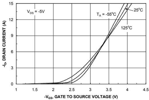
**Figure 5. Transfer Characteristics.**
