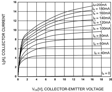
Figure 1. Static Characteristic
