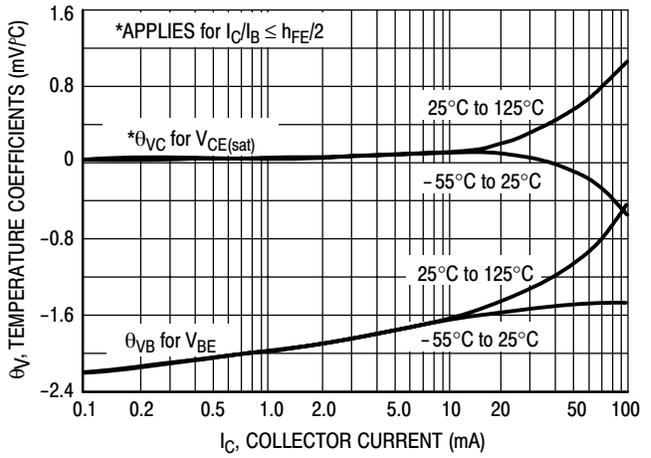
Figure 11. Temperature Coefficients
