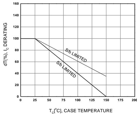
Figure 4. Derating Curve Of Safe Operating Areas
