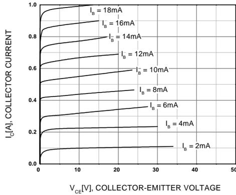
Figure 1. Static Characteristic
