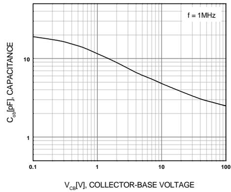
Figure 4. Collector-Base Capacitance
