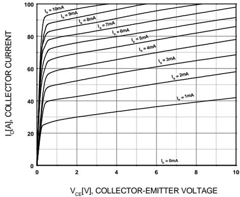
Figure 1. Static Characteristic
