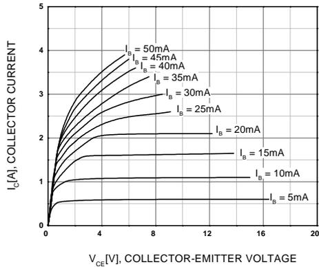
Figure 1. Static Characteristic
