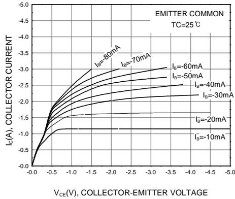
Figure 1. Static Characteristic
