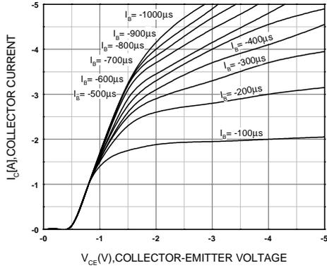
Figure 1. Static Characteristic
