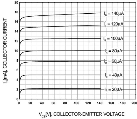
Figure 1. Static Characteristic
