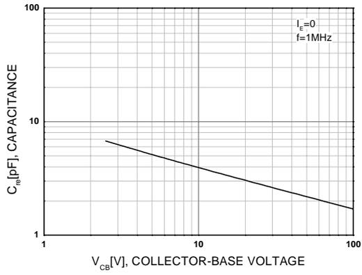
Figure 1. Feedback Capacitance
