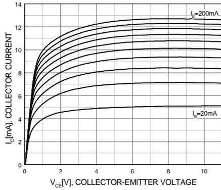
Figure 1. Static Characteristic
