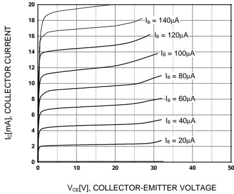
Figure 1. Static Characteristic
