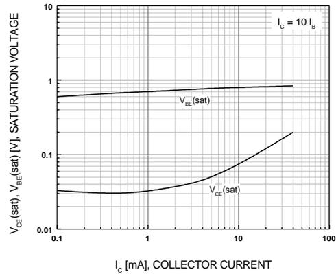
Figure 4. Saturation Voltage
