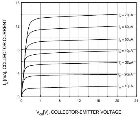
Figure 1. Static Characteristics
