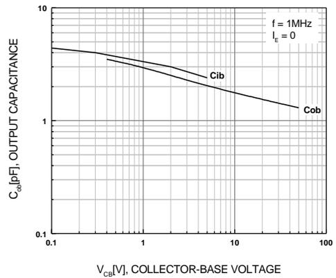
Figure 6. Output Capacitance
