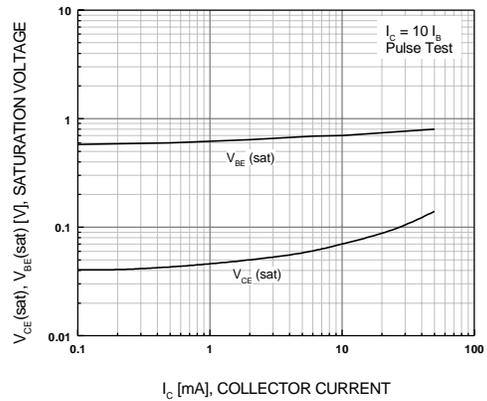
Figure 4. Saturation Voltage
