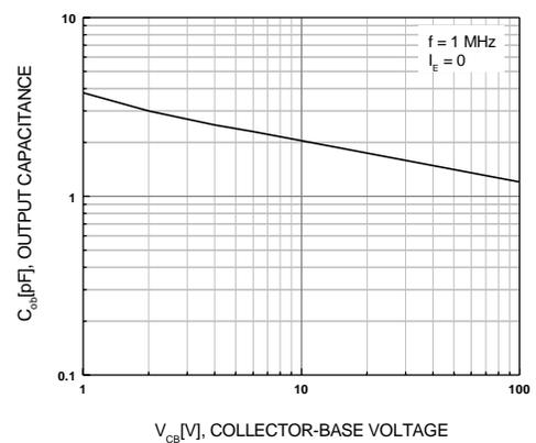
Figure 6. Output Capacitance
