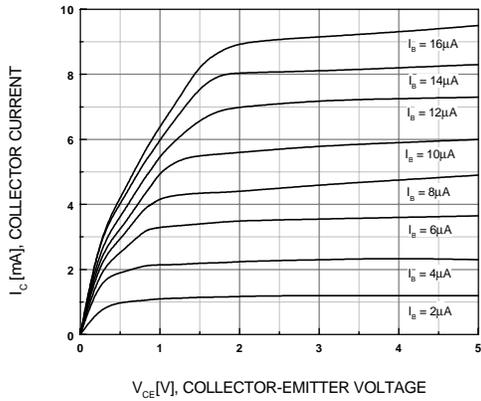
Figure 1. Static Characteristics
