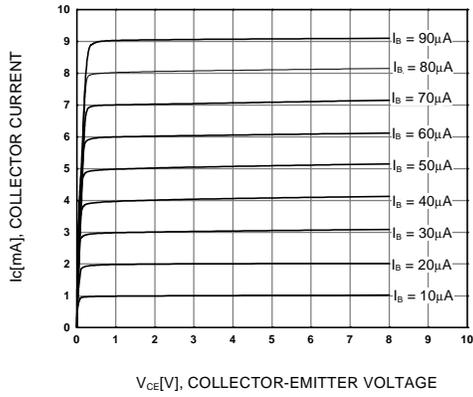
Figure 1. Static Characteristic
