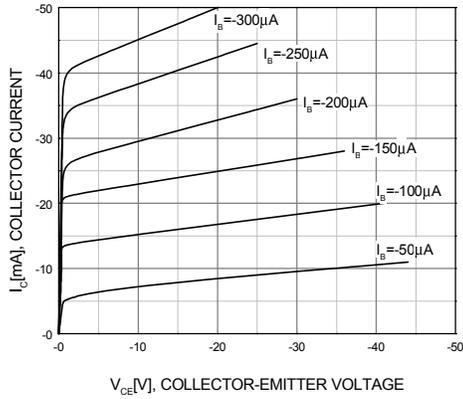
Figure 1. Static Characteristic
