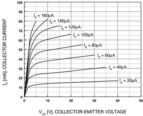
Figure 1. Static Characteristic
