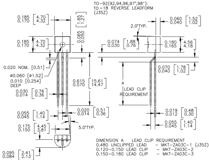
**Note:** All package 97 or 98 transistors are leadformed to this configuration prior to bulk shipment. Order L34Z option if in-line leads are preferred on package 97 or 98.
