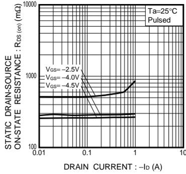
Fig.2 Static Drain-Source On-State Resistance vs. Drain Current
