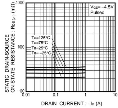
Fig.3 Static Drain-Source On-State Resistance vs. Drain Current
