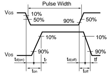
Fig.11 Switching Waveforms
