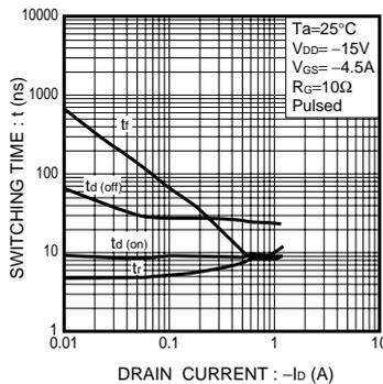
Fig.8 Switching Characteristics
