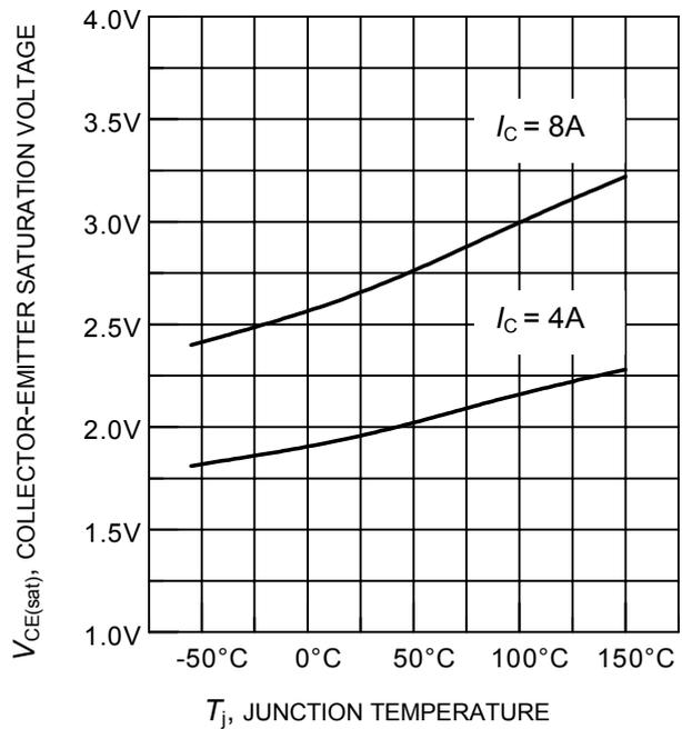
**Figure 8. Typical collector-emitter saturation voltage as a function of junction temperature**
