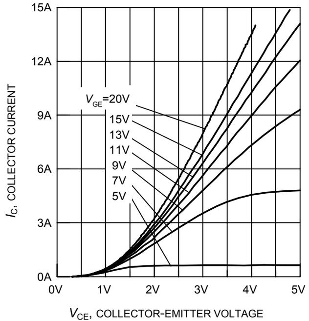
**Figure 6. Typical output characteristics**
