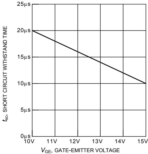
**Figure 19. Short circuit withstand time as a function of gate-emitter voltage**
