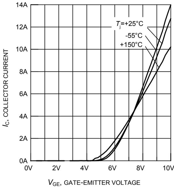
**Figure 7. Typical transfer characteristics**
