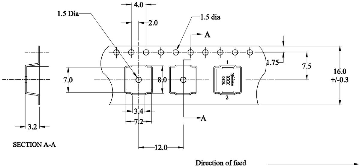
Supplied in tape and reel packaging, 1500 parts per 13" diameter reel.
