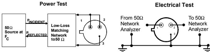
$$CW\ RF\ Power\ Dissipation = P_{INCIDENT} - P_{REFLECTED}$$
